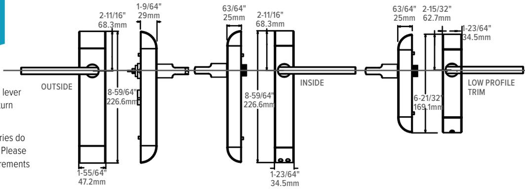
\* The 2190-01, -02, and -03 lever handles are designed to return within 1/2" of the door face.
