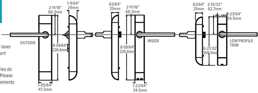
\* The 2290-01, -02, and -03 lever handles are designed to return within 1/2" of the door face.
