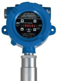
The 5100-28-IT Combustible Gas Sensor Module utilizes infrared sensor technology to monitor for combustible gases (methane and others). Output - Lower Explosive Limit (LEL) or % volume. Explosion proof, Class 1 Div. 1 Groups C, D
