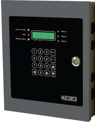
The DVP-120M is a Modbus-Enabled Detection and Ventilation Panel with up to 87 Modbus addressable sensors on three channels of 29 sensors per channel, plus the original 12 analog 4-20 mA sensor channels. The DVP-120M increases the capacity of the DVP-120 from 12 detectors to 99. System wiring includes 4-20 mA current loop and RS-485 serial interface.
