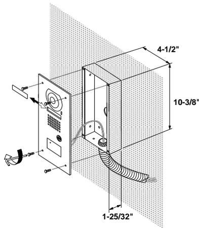
**AX-DVF-P:** Provide a wall surface opening for rough-in backbox (supplied), using dimensions shown.
