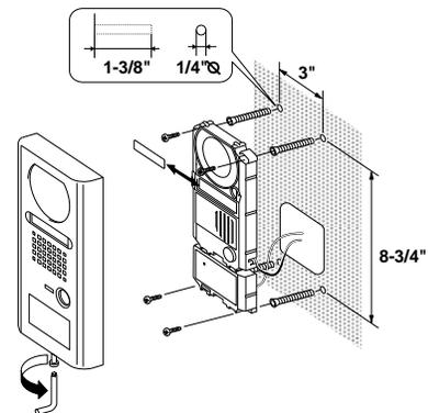
**AX-DV-P:** Provide mounting box or wall opening sufficient for both the CAT-5e cable (from the AX CEU) and the HID card reader wire pigtail.
