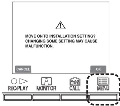
2 Press the [▲], [▼], [◀], and [▶] buttons in the "INSTALLATION" screen to select the item to be set and confirmed, and press the [MENU] button.
