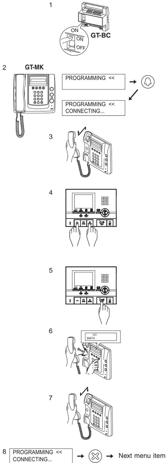
**1** Check that all units are mounted and wired correctly, and then turn on the power switch of the GT-BC.
