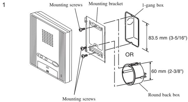
**1** Mount the mounting bracket on the 1-gang box or round back box.
