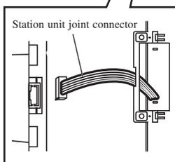
Connect the station unit joint connector.
