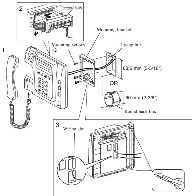
**1** Mount the mounting bracket on the 1-gang box or round back box.
