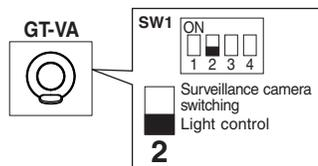
GT-DMV/GT-DM: Enter the program mode and select "LIGHT OR CCTV". Select using the  $\Delta$  and  $\nabla$  buttons.
