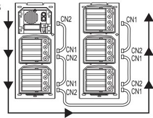
8 Connect the connectors between the modules with cables.
