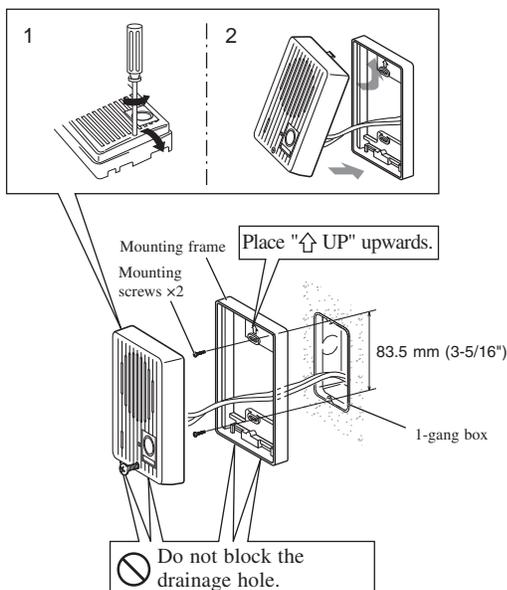
**1** Loosen the screws and remove the mounting frame and main unit.
