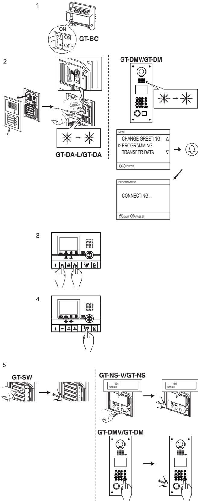
**1** Check that all units are mounted and wired correctly, and then turn on the power switch of the GT-BC.
