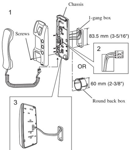
**1** Mount the station unit to the chassis or mounting bracket.
