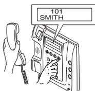
After step 6, press and hold the button until the confirmation tone sounds. A beep will sound and the link to the corresponding residential station will be erased.
