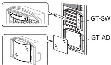
11 For the GT-SW and GT-AD, remove the resident name/address plate or paper by pressing either the left or right end. (Peel off the plastic film.)
