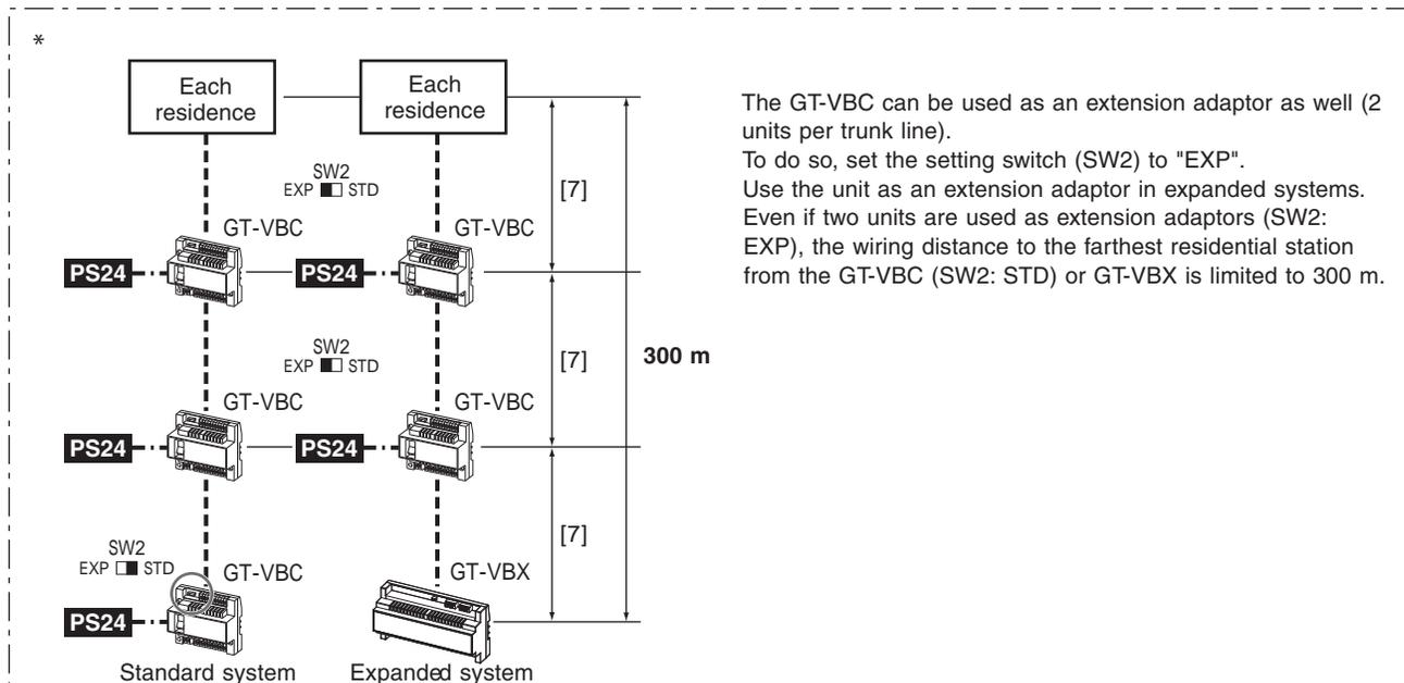
The GT-VBC can be used as an extension adaptor as well (2 units per trunk line).
