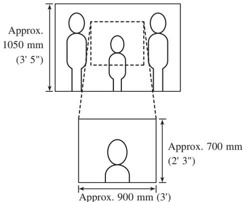
Objects appear smaller due to greater distortion in the surrounding sections compared to the central section, but a wider area is displayed. The display range is a rough estimation and may change due to the installation environment.
