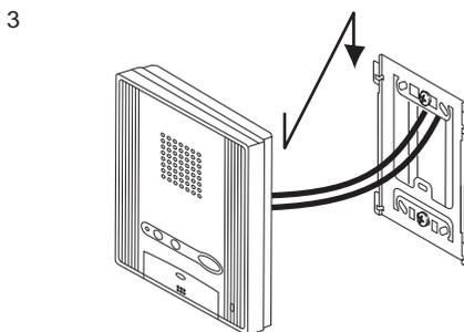
**3** Mount the station unit to the mounting bracket.
