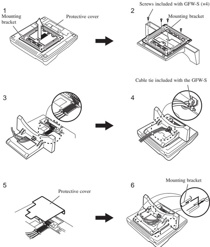
**1** Separate the mounting bracket and the protective cover from the back of the unit.
