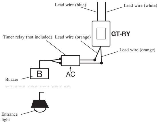
\* When the GT-RY is connected, the separate option connector (4-5) is required.
