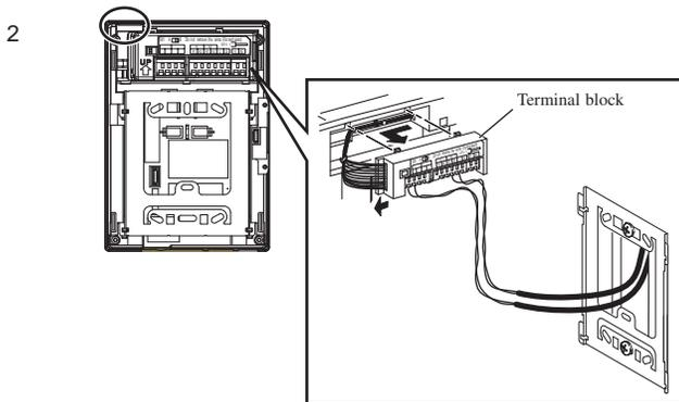
**2** Connect the wiring to the terminal block.
