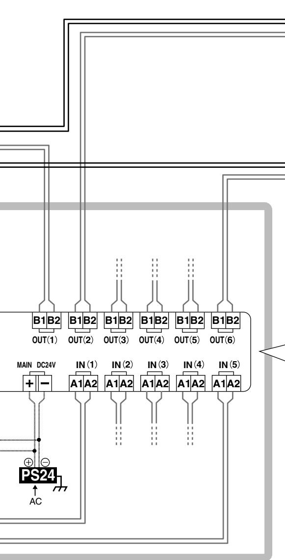
Up to two GT-VBC can be used as extension adaptors per trunk line.
