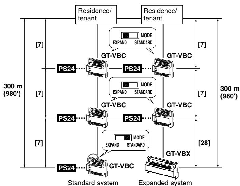
The GT-VBC can be used as an extension adaptor (2 units per sub trunk line).
