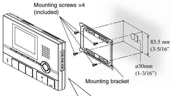
\* When using a gang box, a 3-gang box is recommended.
