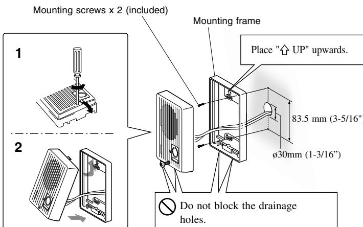
**1** Loosen the screws and remove the mounting frame from the main unit.
