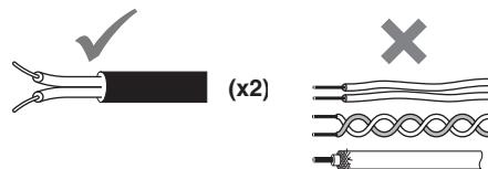
To connect low voltage wires, either crimp them with a crimp sleeve or solder them, and then insulate by covering with insulating tape.
