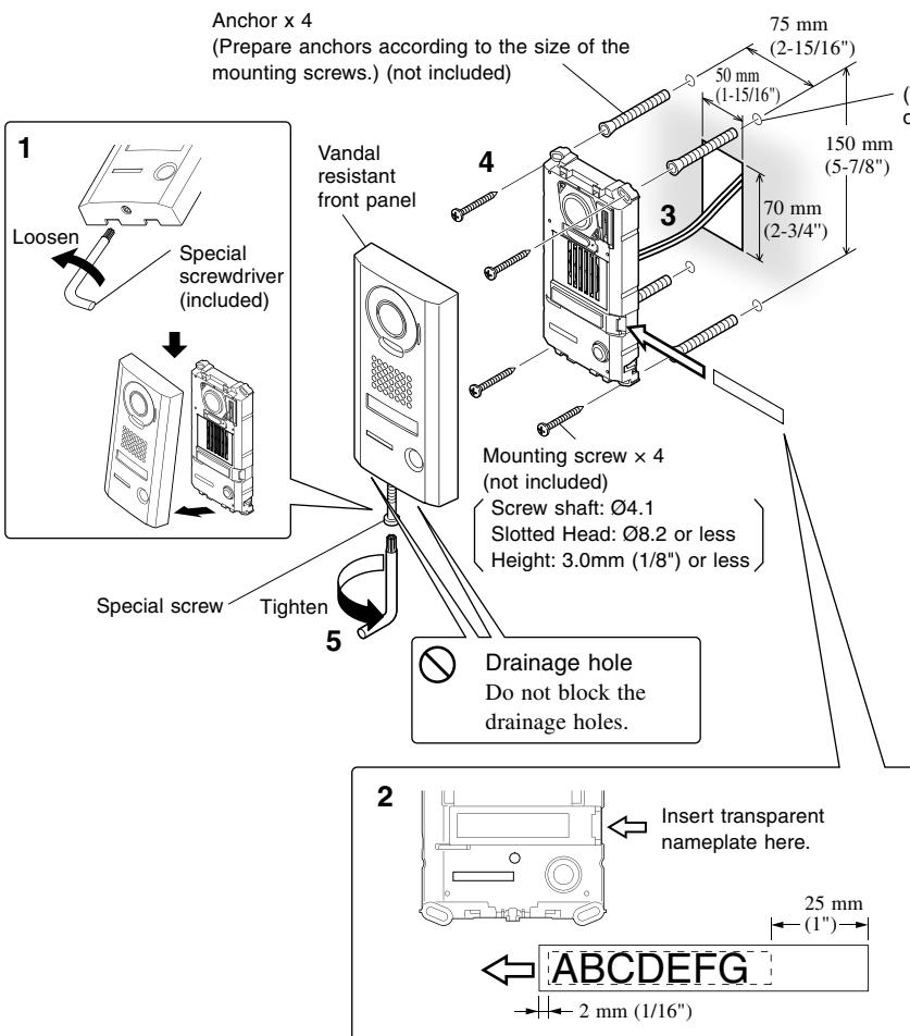
**1** Loosen the special screw with the special screwdriver, and remove the front panel.
