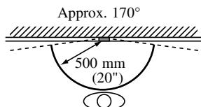
An area over a range of approx. 170° in a 500 mm (20") radius from the camera displays. (The display range is a rough estimation and may change due to the installation environment.)
