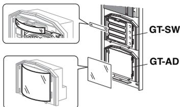
**10** For the GT-SW and GT-AD, remove the resident name/address plate or paper by pressing either the left or right end. (Peel off the plastic film.) Use a permanent pen to write the resident name and address on the transparent plate and mount the plate on the module.
