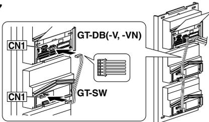
**7** From the audio module to the next module, insert the attached connector into the socket.
