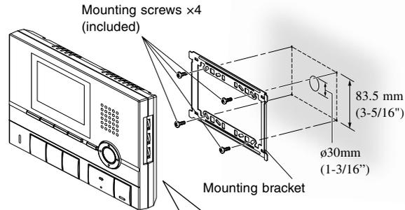
\* When using a gang box, a 3-gang box is recommended.
