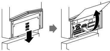
**6** Slide down and then open the terminal cover, and connect wires to the terminal block. Insert the wire into the direct terminal. Press the tab to easily insert the wire into the terminal, then release.
