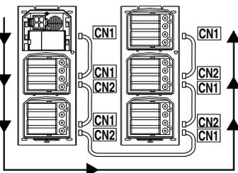
**8** Attach the connection cables between the modules. Mount modules on the back boxes.
