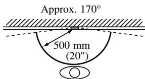
An area over a range of approx. 170° in a 500 mm (20") radius from the camera displays. (The display range is a rough estimation and may change due to the installation environment.)
