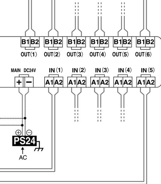
Up to two GT-VBC can be used as extension adaptors per trunk line.
