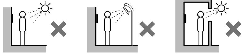
Entrance stations (all-in-one type) include a sensor. Do not place objects such as plants or trees in places monitored by the sensor. Also, placing the unit in bright sunlit areas may prevent the sensor from working properly.
