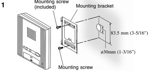
**1** Mount the mounting bracket on the wall.
