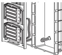
**9** Run the connection cable through the joint pipe and connect CN1 of the GT-SW to the next row.
