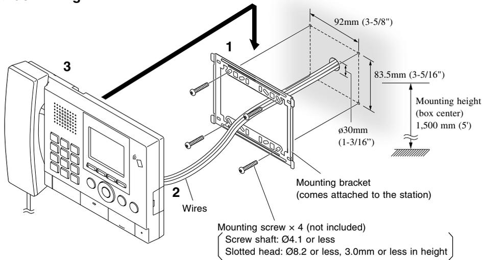
**1** Mount the mounting bracket to the wall.
