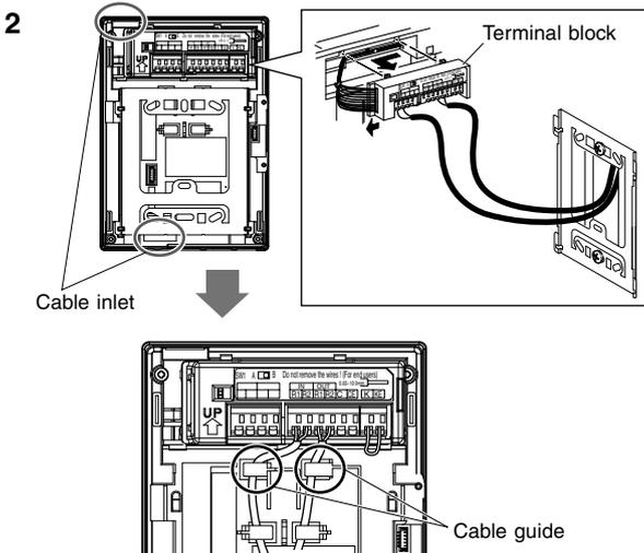
**2** Connect wires to the terminal block.
