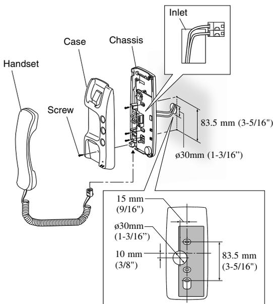
**⚠** Be careful not to damage the circuit board when connecting wires and mounting the station. Failure to do so could damage the station.
