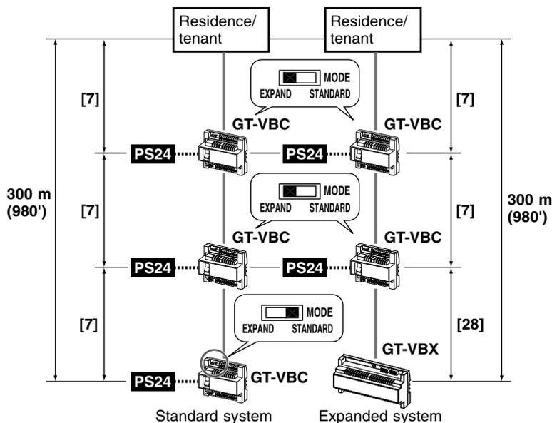
The GT-VBC can be used as an extension adaptor (2 units per sub trunk line). To do so, set the setting switch MODE to "EXPAND". Even if two units are used as extension adaptors (MODE: EXPAND), the wiring distance to the farthest residential/tenant station from the GT-VBC (MODE: STANDARD) or GT-VBX is limited to 300 m (980').
