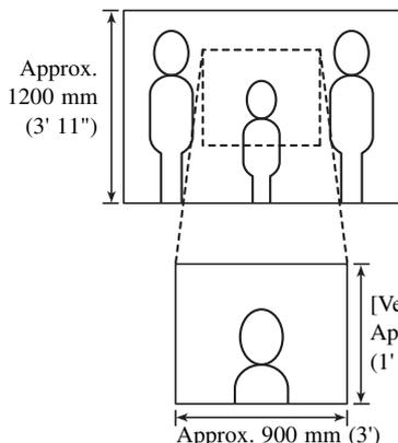
Objects appear smaller due to greater distortion in the surrounding sections compared to the central section, but a wider area is displayed. The display range is a rough estimation and may change due to the installation environment.
