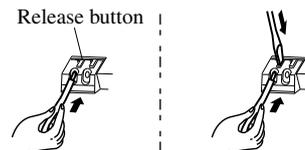
**⚠** Turn off the GT-BC control unit before connecting wires. Failure to do so could damage the station.
