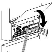
**11** Close the terminal cover. Mount the front frame and tighten with the special screwdriver (included with GT-BC).
