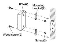
For wall mounting, attach unit to wall with supplied mounting hardware.
