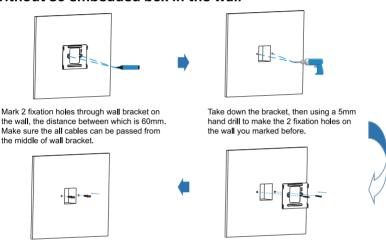
Use 2 ST4X20 screws to fix the wall bracket in the wall.
