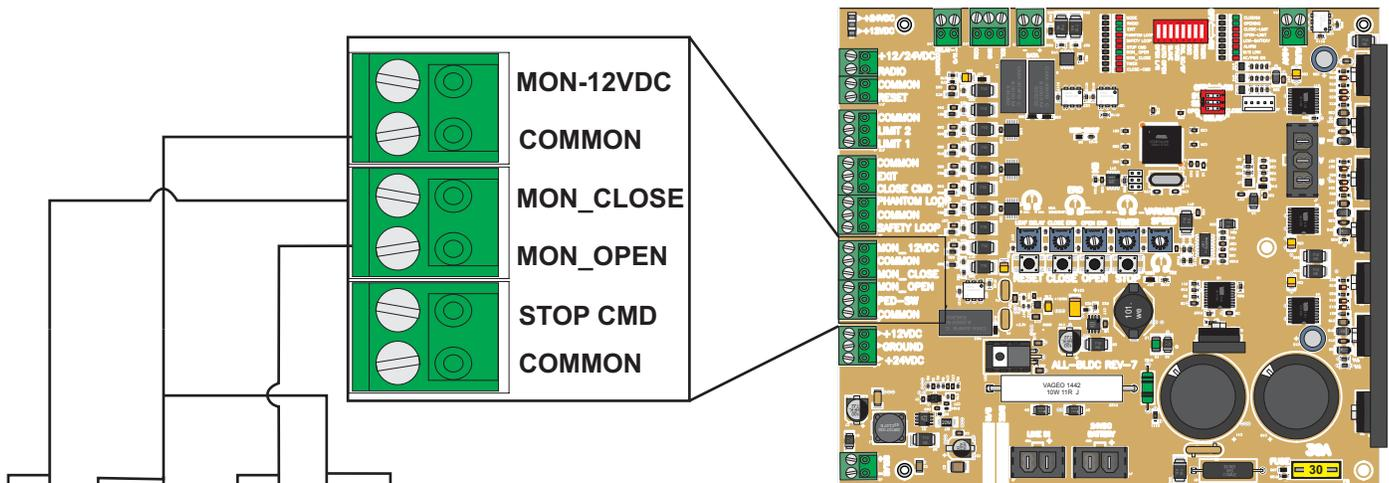
**MON\_CLOSE** (LED will indicate when an obstruction is detected or device is not present)
