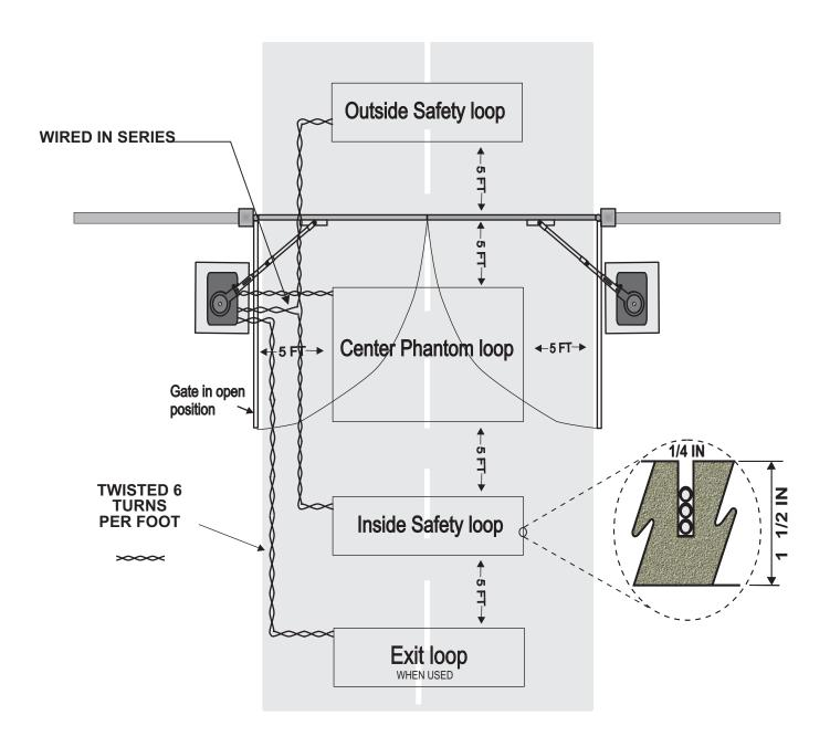
This is a normal loop layout. Remember when connecting to an All-O-Matic circuit board you use the **normally closed contacts** from your safety loop detector and **normally open contacts** from the exit loop. You must twist your wires from your exit point of the saw cut all the way to the circuit board, no exceptions.
