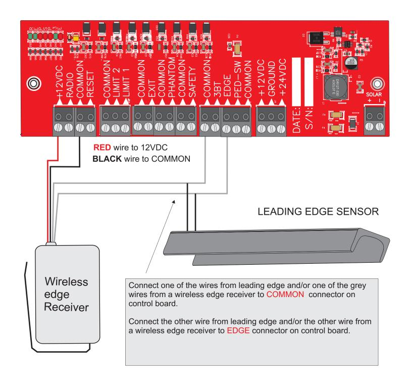
A wireless contact sensor such as one that transmits radio frequency (RF) signals to the gate operator for entrapment protection functions shall be located where the transmission of the signals are not obstructed or impeded by building structures, natural landscaping or similar obstruction. A wireless contact sensor shall function under the intended end-use conditions.
