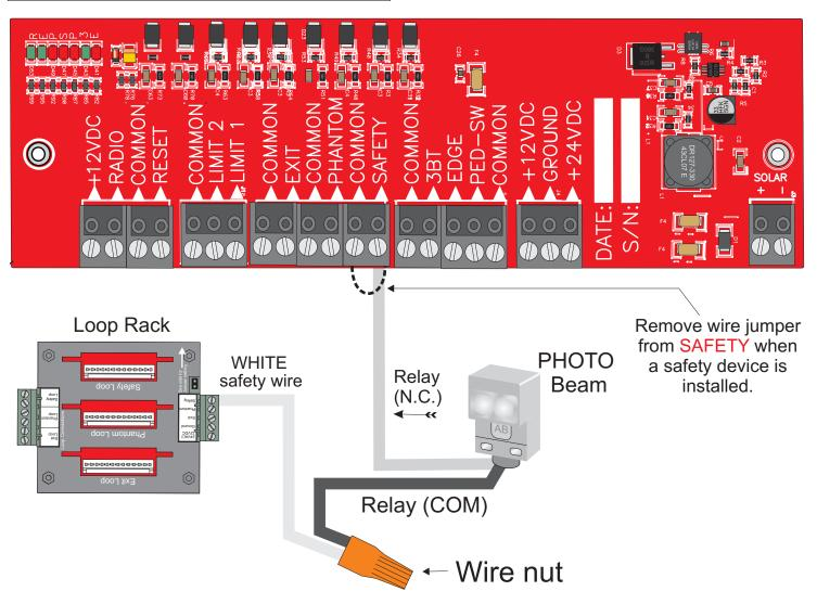
This diagram is for the relay wires of the safety devices, two wires to the board connections (one from each device) and two wires to the orange wire nut.
