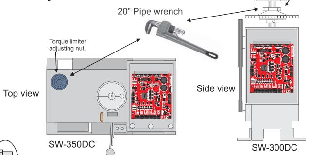
**ARM ADJUSTMENT:** Use a pad lock or a bolt to hold the arm lever in closed position. With the arm lever closed tighten the arm adjusting screw as tight as possible.
