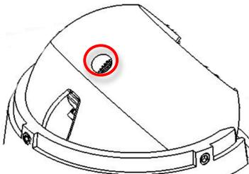
4. Pull the network cable through the ceiling and plug it into the network connector on the camera housing (Note: this can be done at a later time if there is access to the network connector on the camera housing after installation into the ceiling).
