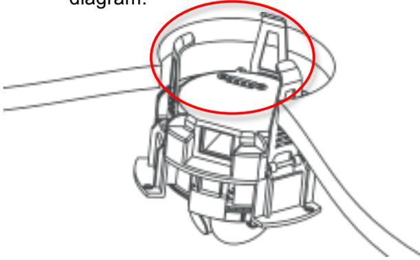
7. Insert the camera housing through the ceiling until the retention arms lock into place.
