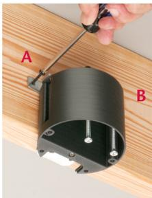
**1** Install FBA426 onto joist with (4) screws: (2) through support tabs (A and B), and (2) more through the front flange.
