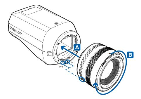
The recommended maximum weight of the lens is 1050 g (2.31 lb). Any lens that is heavier shall be supported by a separate mounting bracket for the lens supplied by the lens manufacturer.
