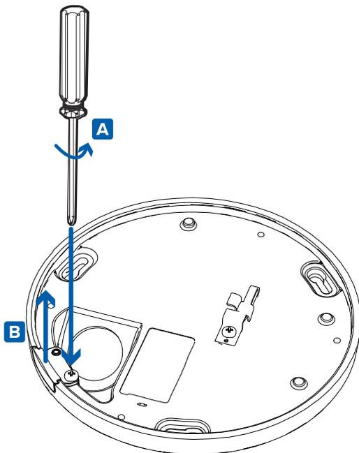
6. Use the same screw to install the optional conduit shroud to the cable entry tab position. The conduit shroud is compatible with up to 1/2" conduits.
