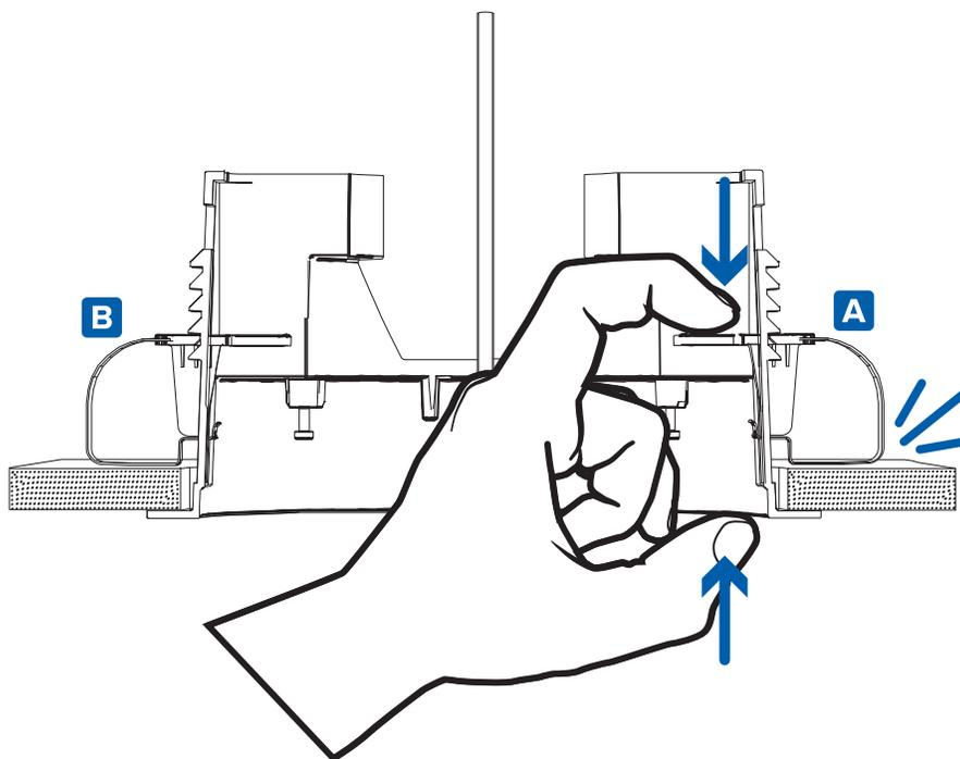
6. Repeat the previous step on the other side. Make sure both clamps are level and horizontal.
