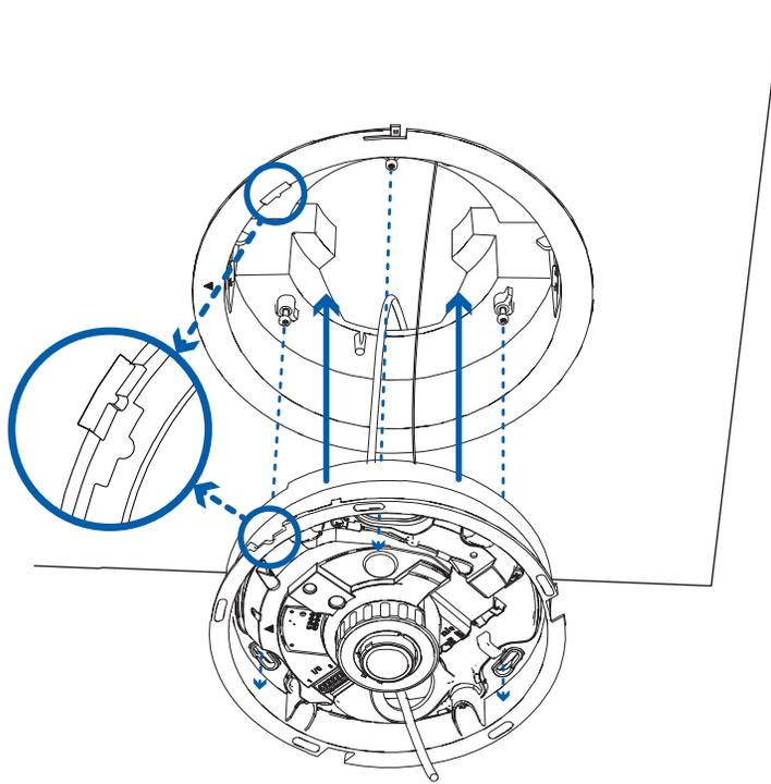
4. Twist the camera base clockwise until the posts come to the right end of the mounting slots and the alignment feature is in the locked position.
