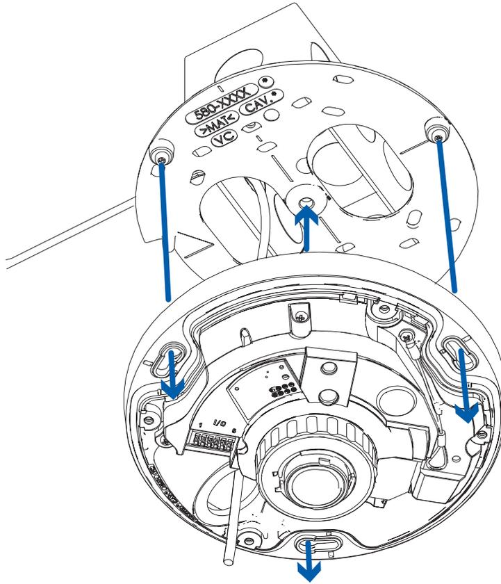
6. Twist the camera base clockwise until the posts come to the right end of the mounting slots.
