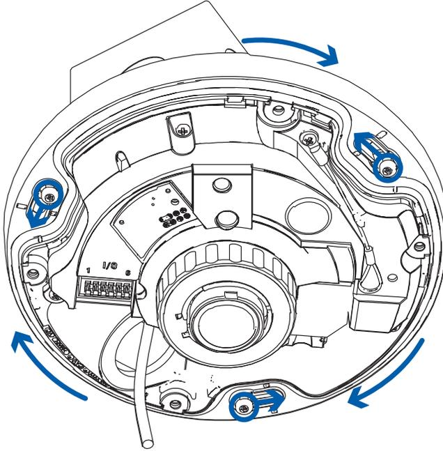
7. Tighten the mounting posts to fix the camera base into place.
