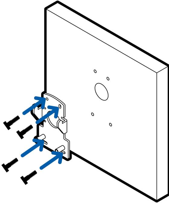
4. Insert the pendant wall mount over the bracket mounting tabs.
