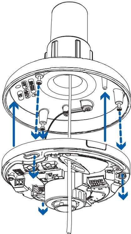
3. Twist the camera base clockwise until the posts come to the right end of the mounting slots.
