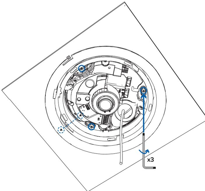
6. Pull the required cables through the rubber sealing grommet. For more information, see *Preparing the Cables* on page 13.
