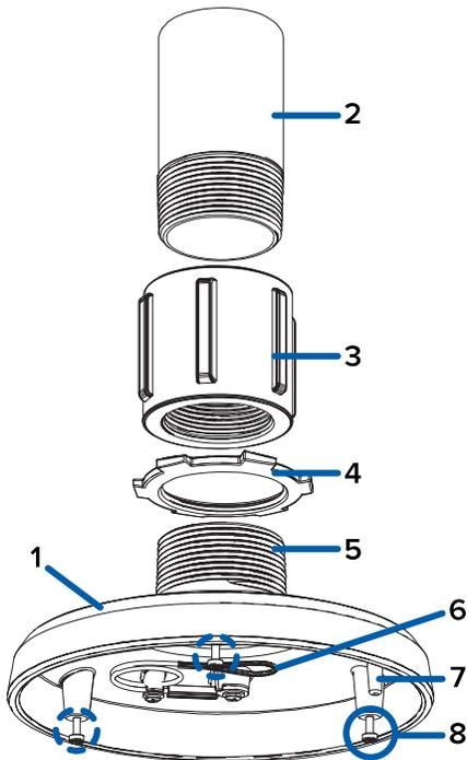
**Note:** The NPT pipe and NPT-female to NPT-female adapter are not supplied by Avigilon and should be sourced separately. However, if you are using the NPT adapter (H5A-FE-MT-NPTA1), the lock nut is included.
