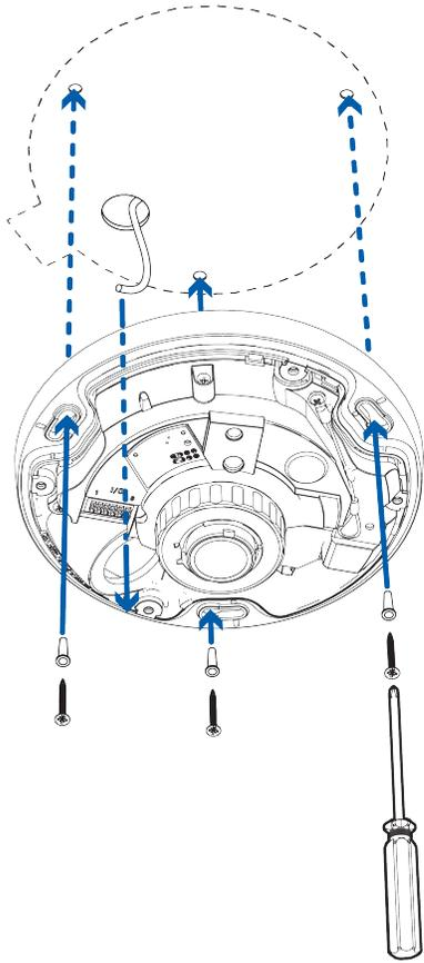
6. Pull the required cables through the rubber sealing grommet. For more information, see *Preparing the Cables* on page 13.
