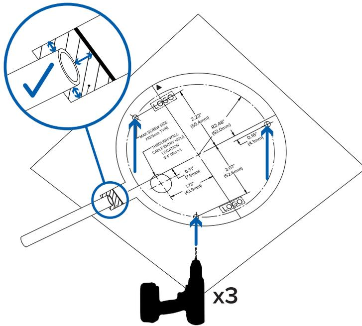
2. Align the conduit for the cables so that the end of the conduit falls inside the conduit landing area of the mounting template.
