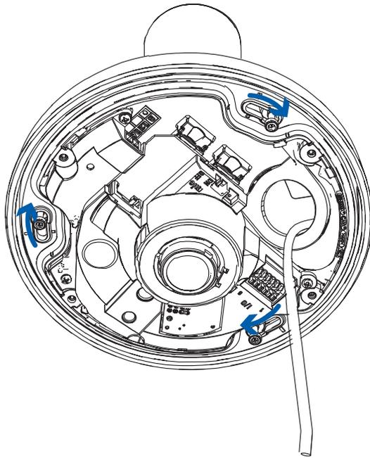
4. Tighten the mounting posts to fix the camera base into place.
