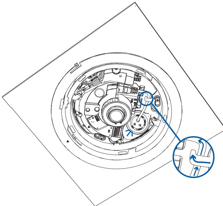
8. Use the cable clip to hold the Ethernet cable in the correct position.
