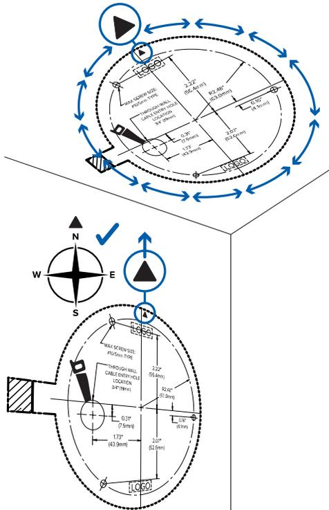
5. Align the up orientation arrow on the camera base with the arrow on the mounting template. Align the mounting slots on the camera base to the drilled pilot holes and use the provided self-tapping screws to secure the camera to the mounting surface.
