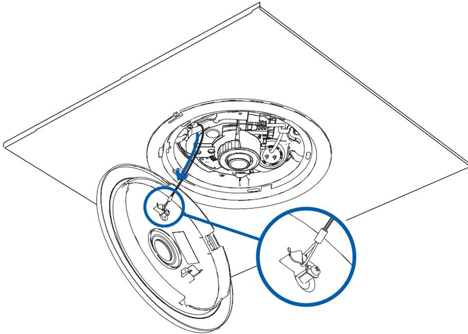
2. Push the in-ceiling cover onto the camera base.
