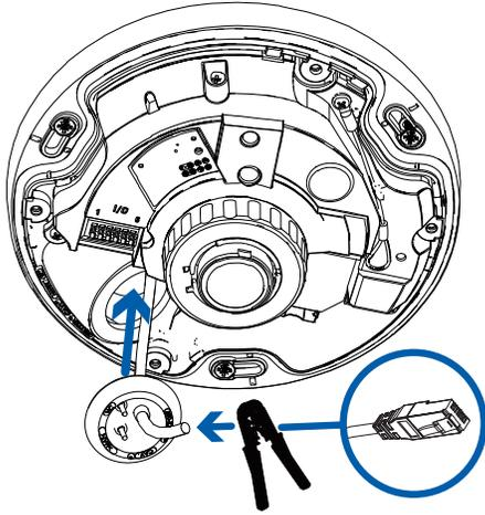
9. Push the rubber sealing grommet with the required cables into the cable entry hole on the camera base. The thread around the grommet should line up with the cable entry hole.
