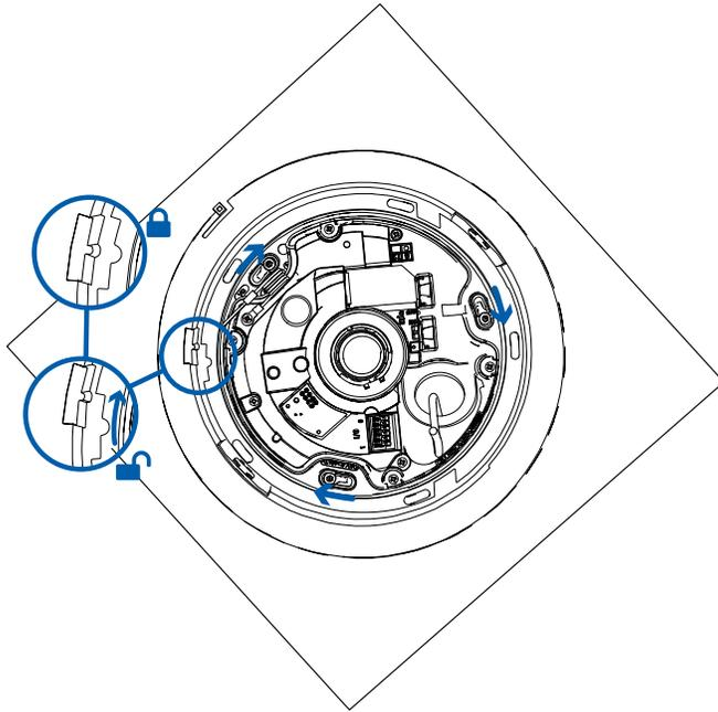
5. Tighten the mounting posts to fix the camera base into place. Ensure that the orientation arrows on the in-ceiling adapter and camera base point in the same direction.
