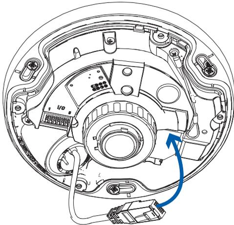
2. If the camera is connected to any external devices, connect the I/O or audio cables to the I/O connector block. For more information, see *Connecting to External Audio and I/O Devices* on page 58.
