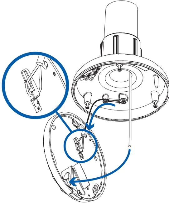
2. Align the mounting slots on the camera base to the mounting posts on the NPT adapter and push the camera base onto the adapter.
