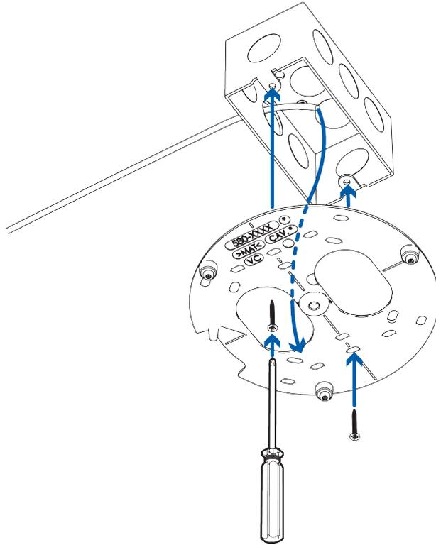
4. Pull the required cables through the electrical box and a cable entry hole on the wall plate. Then feed the cables through the cable entry hole on the camera base.
