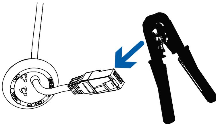
3. If you are using other cables, pull one or both of the tabs on the grommet to open the secondary holes for the additional cables.
