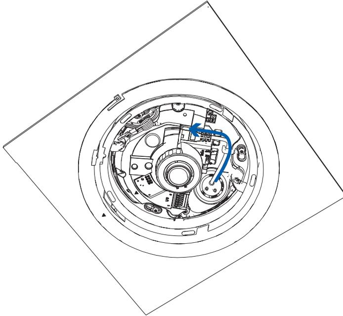
2. If the camera is connected to any external devices, connect the I/O or audio cables to the I/O connector block. For more information, see *Connecting to External Audio and I/O Devices* on page 58.
