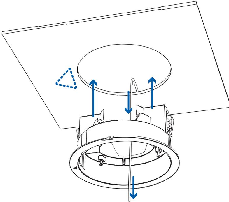
3. Pull off the elastic clamp retainer holding the clamps in place.
