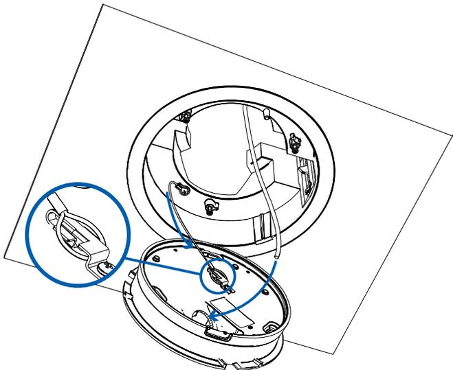
2. Pull the required cables through the cable entry hole on the camera base.
