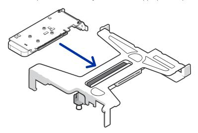
7. Push the expansion card riser back into place and close the expansion card latch.
