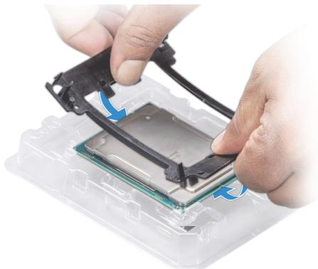
7. Place the heat sink on the processor and push down on the base of the heat sink until the bracket locks onto the heat sink.
