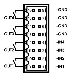
Figure 1: ACC ES 8 Port Appliance I/O pins are numbered as shown in the image above.
