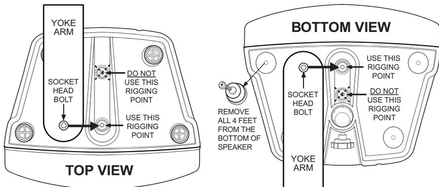
**NOTE:** Be sure to use the Rigging Point which is toward the front of the speaker on both the top and bottom of the speaker enclosure to attach the Yoke socket head bolt.
