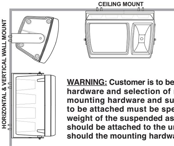
**WARNING:** Customer is to be responsible for the mounting hardware and selection of mounting surface. Both the mounting hardware and surface into which the unit is to be attached must be specified to withstand 10X the weight of the suspended assembly. Also, a safety cable should be attached to the unit so as to prevent from fall should the mounting hardware/surface attachment fail.
