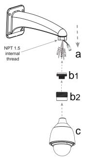
Example installation: AUTODOME IP 5000 HD camera + G 3/4 to M33 adapter + NPT 1.5 to G 3/4 adapter + third-party wall mount
