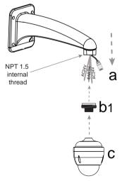
Example installation: AUTODOME IP 4000 HD camera + NPT 1.5 to G 3/4 adapter + third-party wall mount
