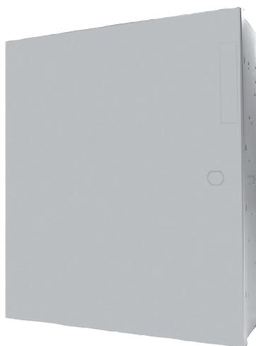
The AE1 is a gray enclosure that accommodates an optional tamper switch for monitoring the door. It is made of 1.0 mm cold-rolled steel and includes a keyed lock. The dimensions are 35.6 cm x 31.8 cm x 7.6 cm (14 in. x 12.5 in. x 3 in.).
