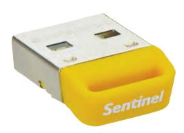
The D5371-USB is a required accessory for RPS-LITE. Without it, communication with the control panel is not possible. It is plugged into the computer's USB port and is color-coded yellow.
