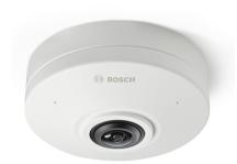
The FLEXIDOME panoramic 5100i is a discreet and aesthetic panoramic camera for indoor surveillance. Its stereographic, panoramic lens provides full 360° coverage without blind spots, ideal for surveillance applications that require wide area coverage in a single, detailed view. The camera offers full situational awareness and simultaneous high-resolution zoomed-in images. The high-end system on chip (SoC) provides dewarping for easy integration and flexible viewing and recording.
