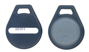
Randomly-coded, gray, plastic, token that attaches to a key chain. It works with D8223, D8223-P, D8224, D8224-SP, and D8225 Proximity Readers. The token is Wiegand 26-bit. Each package contains ten tokens.
