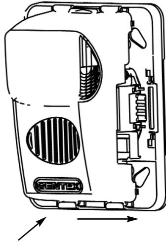
Candela selection slider switch. Depress center and slide switch to desired brightness level.
