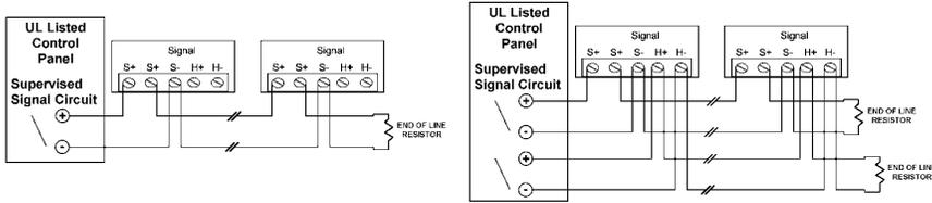
MAX. WIRE DISTANCE (IN FEET) =  $\frac{(\text{PANEL VOLTAGE} - \text{APPLIANCE MIN. VOLT}) \times \text{WIRE CONDUCTIVITY}}{\text{TOTAL CURRENT DRAW}}$
