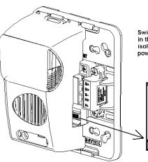
Switch positions 1 and 2 in the off position to select isolated horn and strobe power inputs.
