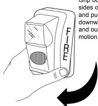
Grip both sides of bezel and pull in a downward and outward motion.
