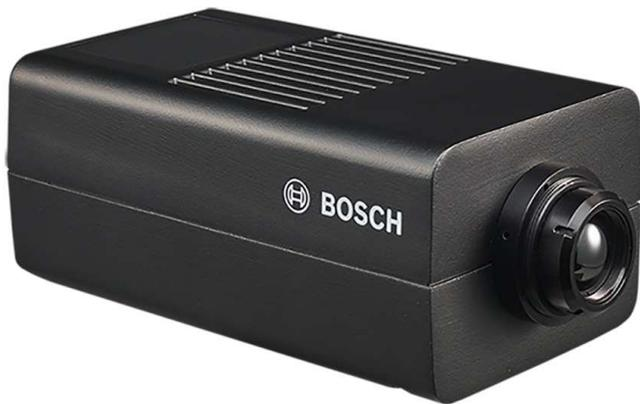
The DINION IP thermal 9000 RM camera, based on an un-cooled vanadium oxide microbolometer, is a contactless tool to measure surface temperature at short range. The camera has a QVGA sensor with a frame rate of 9 FPS.
