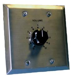
The Cooper Wheelock SAFEPATH4 SP-SVC Supervised Volume Control is used with the SP40/2 or SP40S Facility Communications Systems along with the SPB-80/4, SPB-160, or SPB-320 Audio Power Boosters to control the volume of a single speaker, multiple speakers, or an entire audio loop up to 35 W. An integrated override relay bypasses the volume attenuator in alarm conditions allowing the emergency notification message to be announced at maximum volume.
