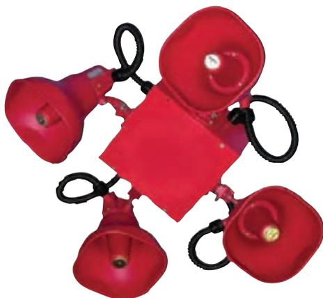
The Wheelock STH Series Cluster Horn Loudspeakers are designed for high ambient noise environments such as manufacturing plants, processing plants, and factories. They are available in configurations with two, three, or four horns that meet the requirements of UL1480. Each horn can deliver up to 102 dB at 15 W at 10 ft (3 m).
