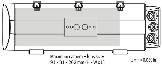
Dimensions in mm for all models, maximum internal usable space available (based on camera/lens size)
