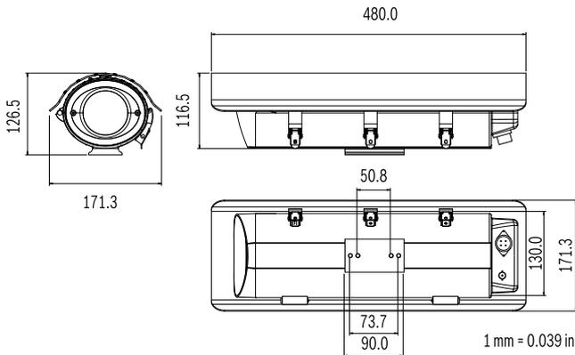
Dimensions in mm for UHO-HBPS-10, UHO-HPS-50 and UHO-HBPS-50 housings outdoor units
