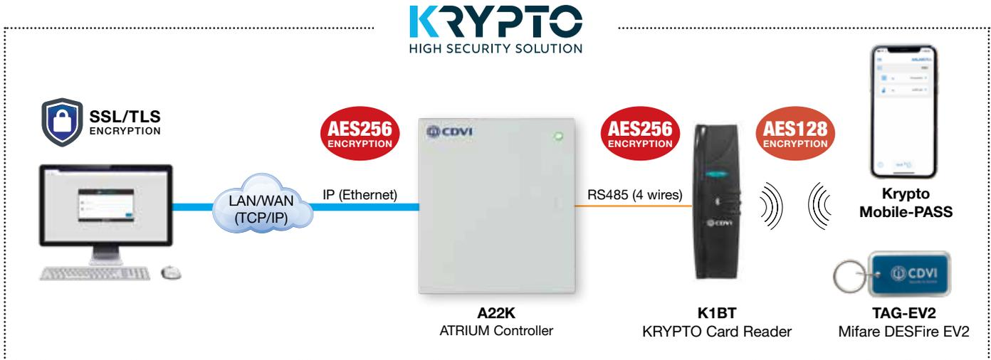
Supports any combination of fifty A22K, A22KEC and/or ADH10K controllers for a maximum of 500 doors
