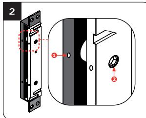
Insert the cable of the magnet. Unfasten the screws on the side of the armature plate (1) with the Allen key. Mount temporarily the CZ3000. Then adjust the gap between the magnet and the armature plate by adjusting the top screws on the armature, allow 2mm distance maximum. Tighten the 2 screws on the side of the armature plate (2) once the test on magnet has been successfull.
