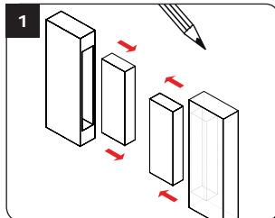
Make a cut on the door leaf and a cut on the door jamb in order to insert the magnet and the armature plate of the CZ3000 magnet. Then mark the mounting holes of the mounting screws. Drill the mounting holes of the magnet and of the armature plate in order to facilitate the screwing. Drill the cable access hole.
