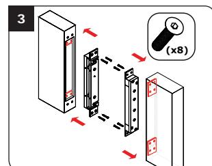
Place the magnet on the back plate of the surface housing as well as the armature on the second back plate of the surface housing and fasten definitely the magnet on the door.
