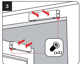
Fasten definitively the magnet on the door and place the housings.
