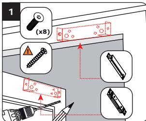
Measure and mark the center lines to determining the magnet position on the jamb and the armature plate on the door leaf frame. Then drill the fixing screw holes to fasten the screws easily.
