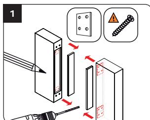
Make a cut on the door leaf and a cut on the door jamb in order to insert the magnet and the armature plate of the CZ3000 magnet. Then mark the mounting holes of the mounting screws and drill the mounting holes of the magnet and of the armature plate in order to facilitate the screwing.
