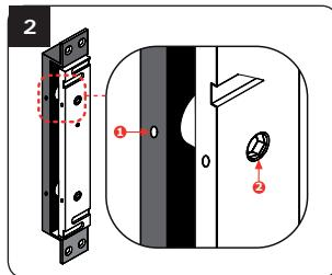
Mount the brackets of the housing on the jamb and on the door leaf. Insert the cable and fasten temporarily the magnet and the armature plate to the bracket of the housing. Unfasten the screws on the side of the armature plate (1) with the Allen key. Then adjust the gap between the magnet and the armature plate by adjusting the top screws on the armature, allow 2mm distance maximum. Tighten the 2 screws on the side of the armature plate (2) once the test on magnet has been successfull.
