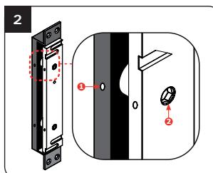
Mount the back plate of the housing (note that the screws are not included). Unfasten the screws on the side of the armature plate (1) with the Allen key. Mount temporarily the CZ3000. Then adjust the gap between the magnet and the armature plate by adjusting the top screws on the armature, allow 2mm distance maximum. Tighten the 2 screws on the side of the armature plate (2) once the test on magnet has been successfull.
