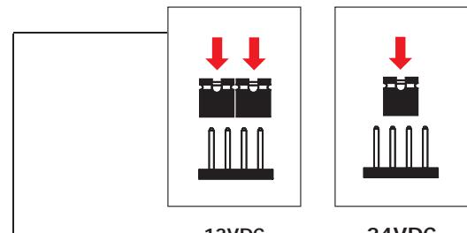
\* **Input voltage: 12 VDC or 24 VDC**
