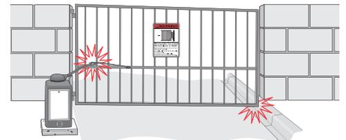
The gate hits the driveway, curb or other, and gets stuck or bent in an awkward position.
