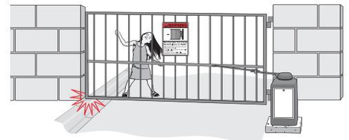
A foreign object is on the gate frame while the gate is moving.
