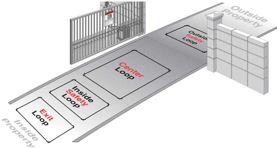
**110Vac "Center" Loop Detector:** Allows gate to stay open when vehicles are obstructing path. Caution: This option is for all vehicles including ones less than 14 feet long. Center loop system requires two safety loops.
