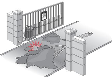
An externally wired photoelectric sensor has been triggered twice (photoelectric sensor blocked).
