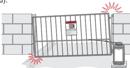
Gate hinges are too tight or broken and the gate is not moving freely.
