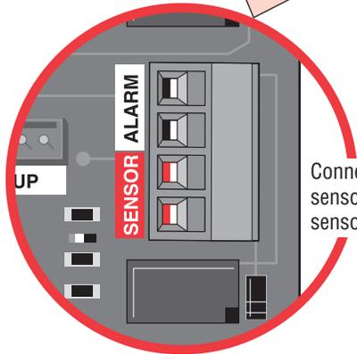
Connect both edge sensors parallel to sensor connector.
