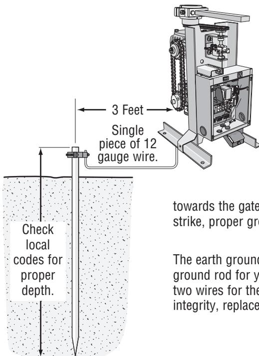
Proper grounding gives an electrical charge, such as from an electrical static discharge or a near lightning strike, a path from which to dissipate its energy safely into the earth.
