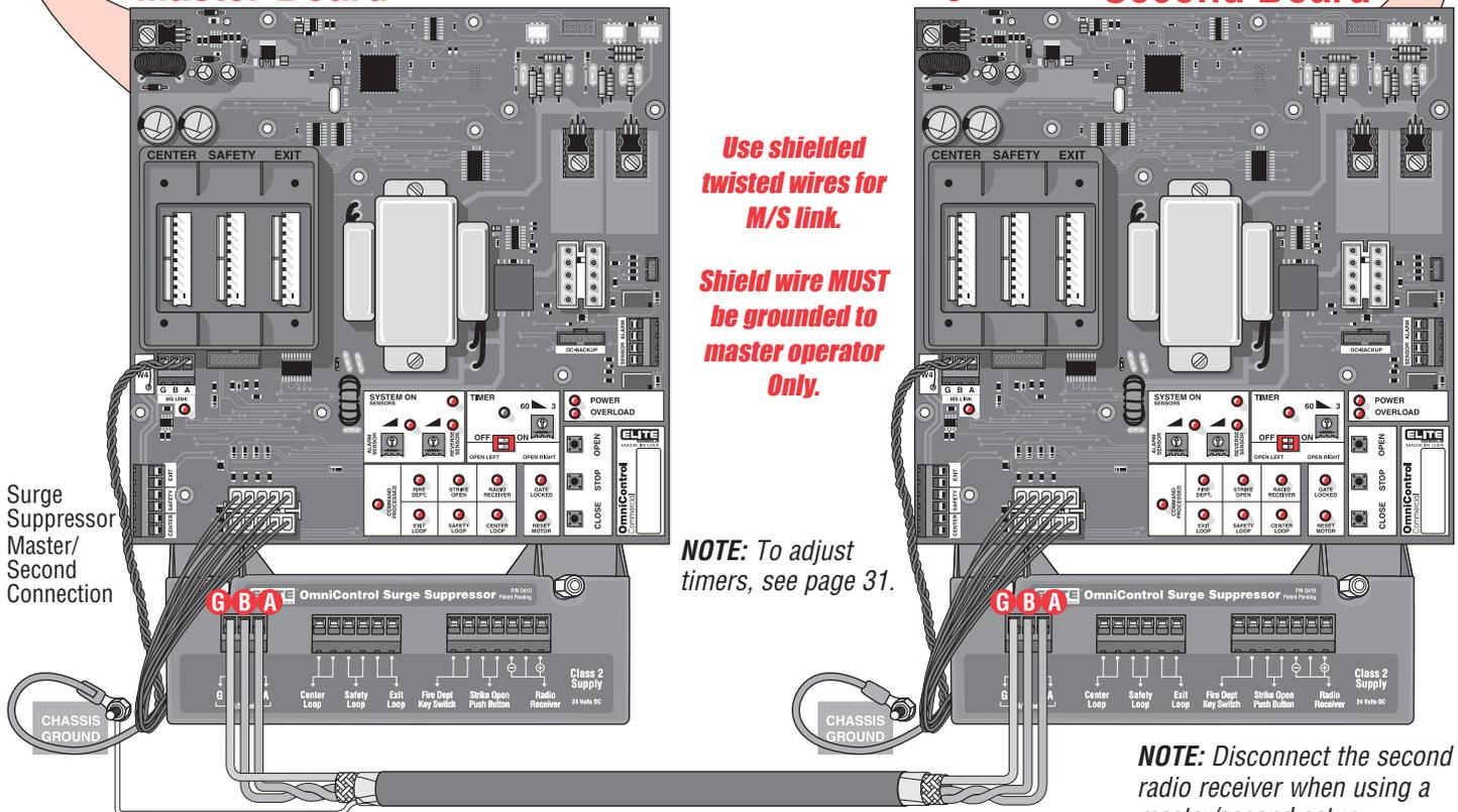
Use shielded twisted wires for M/S link.
