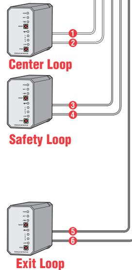
**NOTE:** Use separate 110Vac power for each loop detector.
