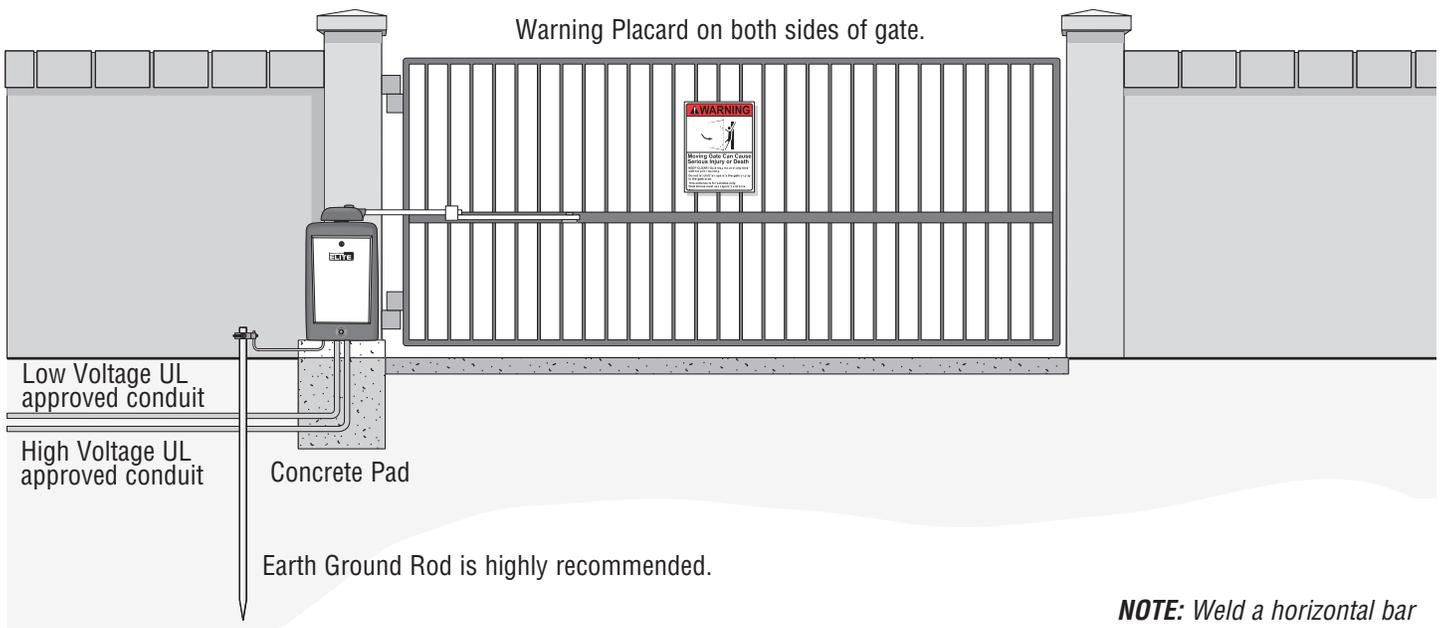
**NOTE:** Weld a horizontal bar across entire gate on any installation for strength.
