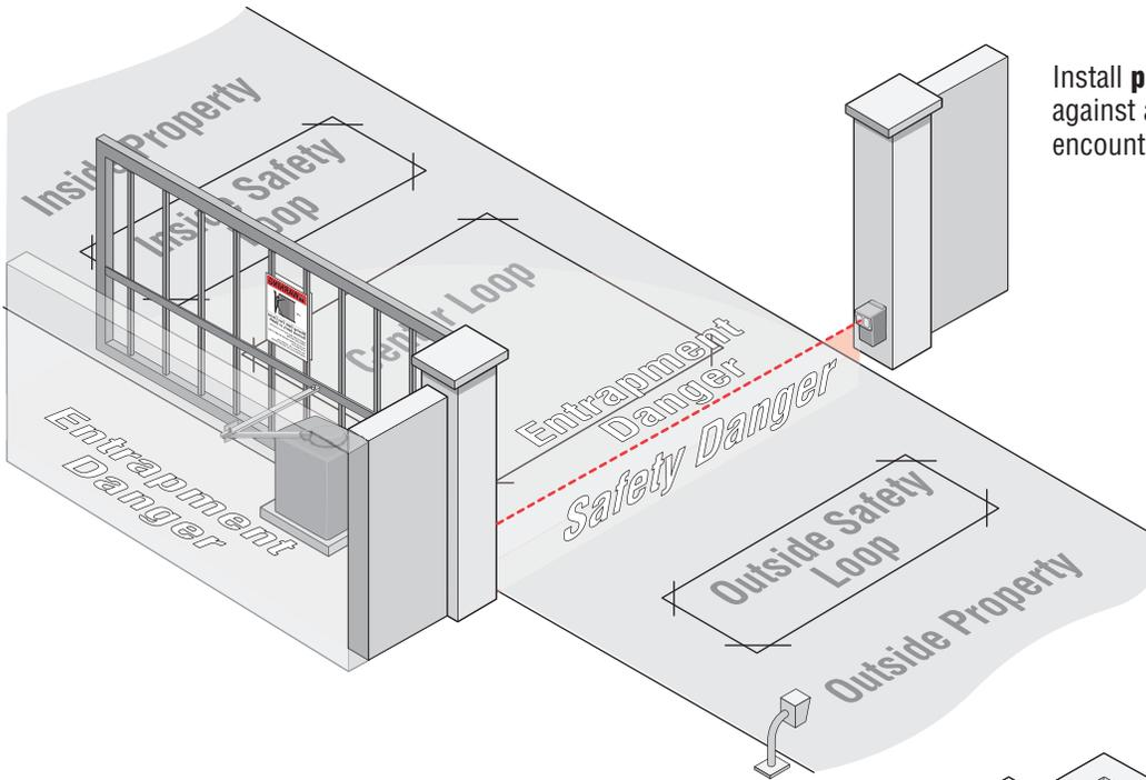
Install **photoelectric sensors** to protect against any entrapment or safety conditions encountered in your gate application.
