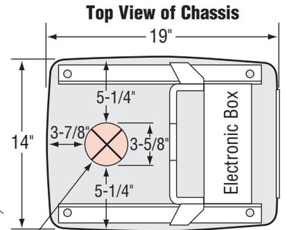
Approximate placement of high voltage and/or low voltage conduits.
