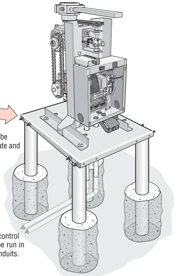
Power and control wiring can be run in separate conduits.
