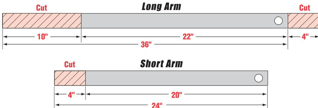
Follow the exact measurements, then cut the standard arm to meet the shorter measurements.
