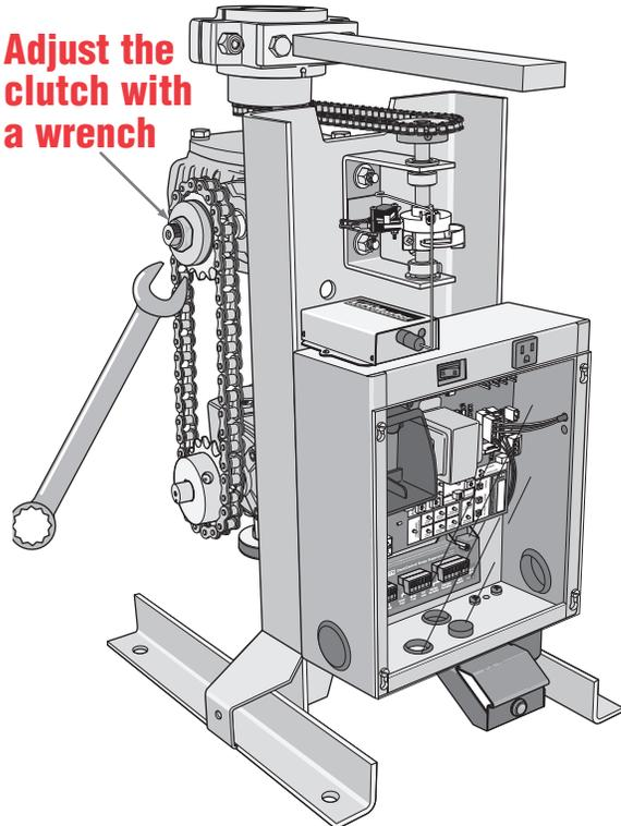
**Adjust the clutch with a wrench**
