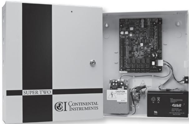
The two-reader Super-Two (CICP-1300) supports 2 readers and has 8 inputs, 1 tamper alarm and 5 relay outputs. A locking steel enclosure, power supply and 7AH battery are included. Plug-in network interface, memory expansion, X-Y matrix keypad support and input/output expansion are optional. In addition to power for the controller and two readers, 1.2A at 12VDC is provided for accessories, including power strikes and mag-locks.
