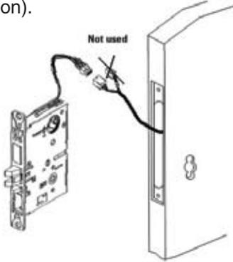
For non ElectroLynx Connector System, door install available retrofit harness and use with ElectroLynx hinge. Follow installation instructions for ElectroLynx Connector System.
