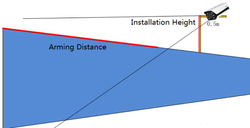
When installing cameras on the perimeter, there might be blind area, and you can install two cameras face to face to realize monitoring without blind area.
