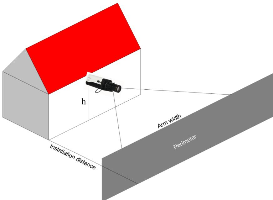
Install cameras using the following suggestions. Note that a shorter installation distance translates to a smaller monitoring area.
