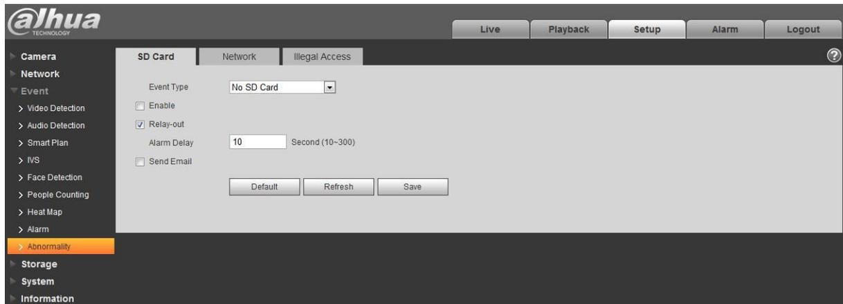
5. Select the event from the Event Type pull-down menu (No SD Card, Capacity Warning, SD Card Error).
