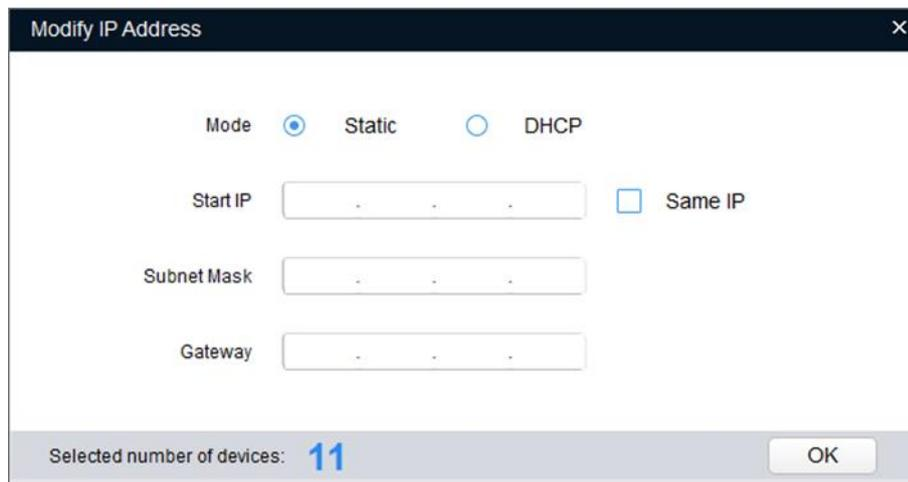
Step 3 Select **Static** mode, and then enter start IP, subnet mask, and gateway.
