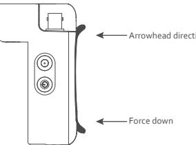
The wristband quickly disassembles from the tester. Press and hold the disassembly button at the bottom of the tester, and lift it up to separate the wristband from the tester.
