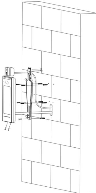
**Step 5** Make the cable connections. Refer to Section 2.3 Cable Connections, for more information.
