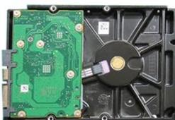
4. Align the four screws in the HDD casing with the holes on the bottom of the NVR. Place the HDD into the NVR housing.
