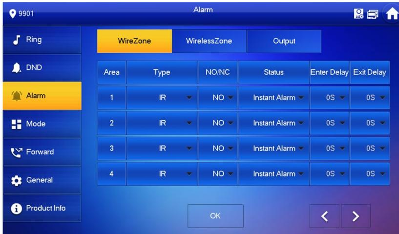
4. Press a corresponding position to set area type, NO/NC, alarm status, enter delay, and exit delay.
