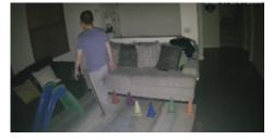
**Smart Illumination mode:** White light LED triggered only when a person is detected. Remain IR mode otherwise for power saving and less disturbance.
