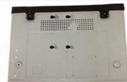
6. Turn the DVR over and connect the SATA cable and the power cable to the HDD. You can connect the HDD data cable and the power cable first and then fix the HDD in the device.
