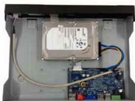
7. Align the upper housing with body of the DVR, then push the clips in and then place the cover back onto the DVR.
