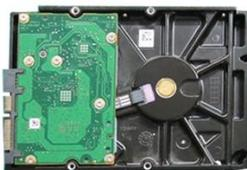
4. Align the four screws in the HDD casing with the holes on the bottom of the DVR. Place the HDD into the DVR housing.
