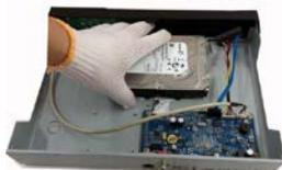
5. Turn the DVR upside down and then firmly tighten each screw to secure the HDD to the DVR.
