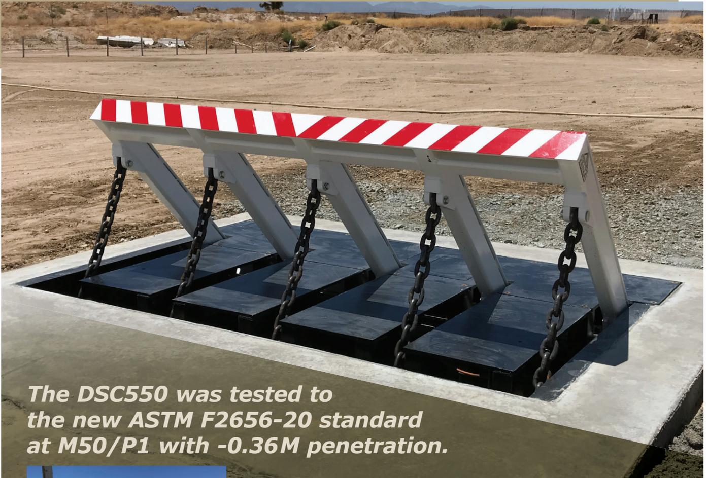
*The DSC550 was tested to the new ASTM F2656-20 standard at M50/P1 with -0.36M penetration.*
