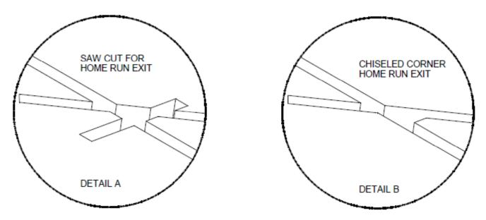
Once the saw slot has been cut, the slot should be cleaned of all loose material. High pressure air should be directed in to the saw slot to remove all debris. This will also help remove dust from the saw cutting operation from the sides of the saw slot. This will allow better adhesion of the loop sealant to the saw slot.
