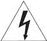
The lightning flash with arrowhead symbol, within an equilateral triangle, is intended to alert the user to the presence of dangerous voltage within the products enclosure that may be of sufficient magnitude to constitute a risk of electric shock to persons.
