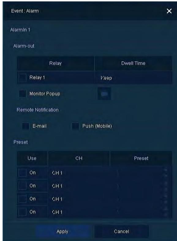
Figure 4-28 Event > Alarm In > Setup > Event: Alarm
