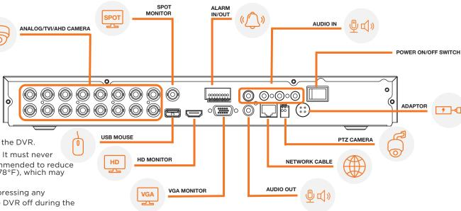
To prevent the DVR from overheating, do not operate it in an area that exceeds the maximum recommended ambient temperature of 104°F (40°C). To prevent airflow restriction, allow at least 3 inches (7.6 cm) of clearance around the ventilation openings.
