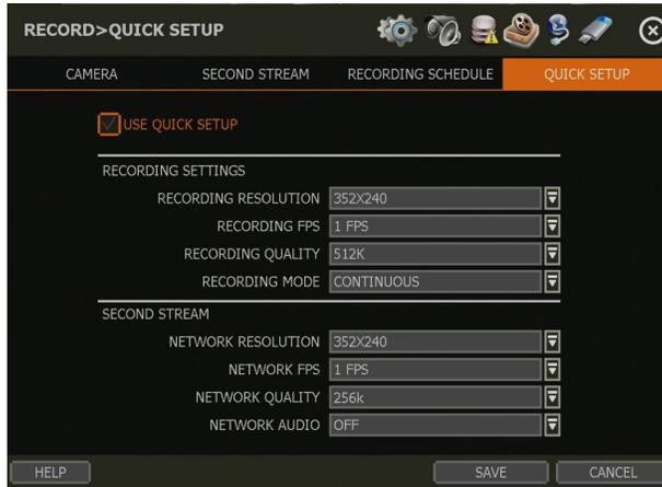
User can setup recording resolution, FPS, quality and mode on recording settings. And user can also setup network resolution, FPS. Quality and audio on second stream setting.
