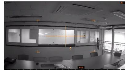
**NOTE** Full PTZ functions are available by using the USB mouse, IR remote control, or keyboard controller. Availability of functions depends on the camera. Consult the camera's manual for more information.
