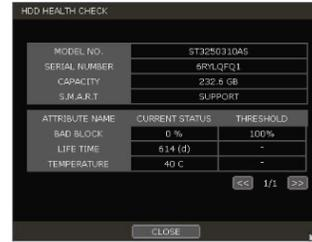
**WARNING** To achieve high-level system stability, warning message of high temperature will pop up when temperature inside the system exceeds optimum range. This problem may be driven from malfunction of ventilation fans. Inspect if the cooling fan is properly working, or temperature around the system is properly kept.
