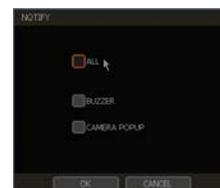
**Note** “Camera pop-up” means that multi-screen live video mode will be switched to single channel mode automatically upon alarm triggered. This single channel video is the channel triggered by alarm.
