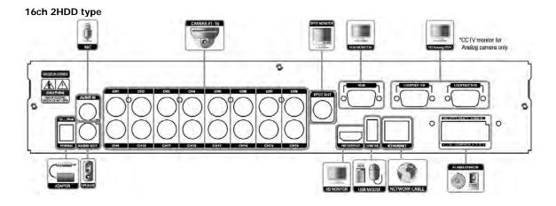
WARNING! \*When connecting power cord to the system, it is strongly recommended first to plug the power cord to the system and then plug the other side of power cord into the wall socket.
