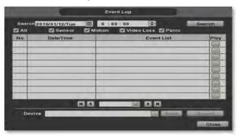
Note If an alarm or event do not appear in the envent log, check the alarm settings, and connection port at the DVR's rear panel.
